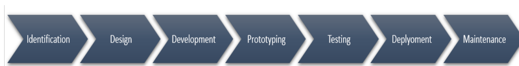
Figure 1. Mobile Application Development Life Cycle (MADLC) phases
